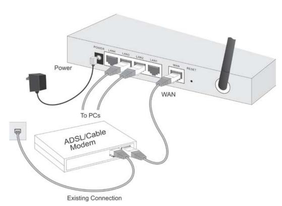
Figure 3: Installation Diagram
